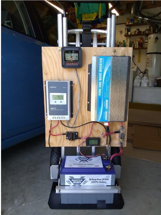
Portable Battery Storage Unit
